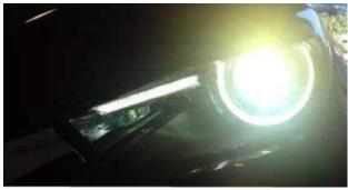
This is a common condition on headlights using a white LED light source. With a present production technology of white LED and optical construction of headlights, it is difficult to eliminate light color differences of LED headlights completely.
